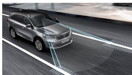
Illustration of camera detection used in Lane Keep Assist technology
